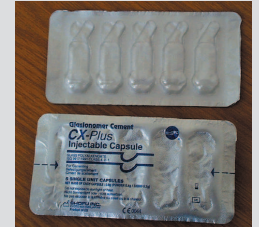
Sample of a medicine packaging made of aluminium/PE
